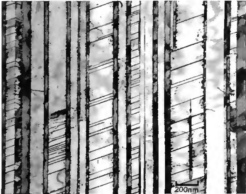
Figure 4.22: Deformation in the fine lamellar regions which is concentrated in the \gamma phase. Note that for the lamellae with the same orientation as B ( Fig 4.18 ) only one twinning system is active.
