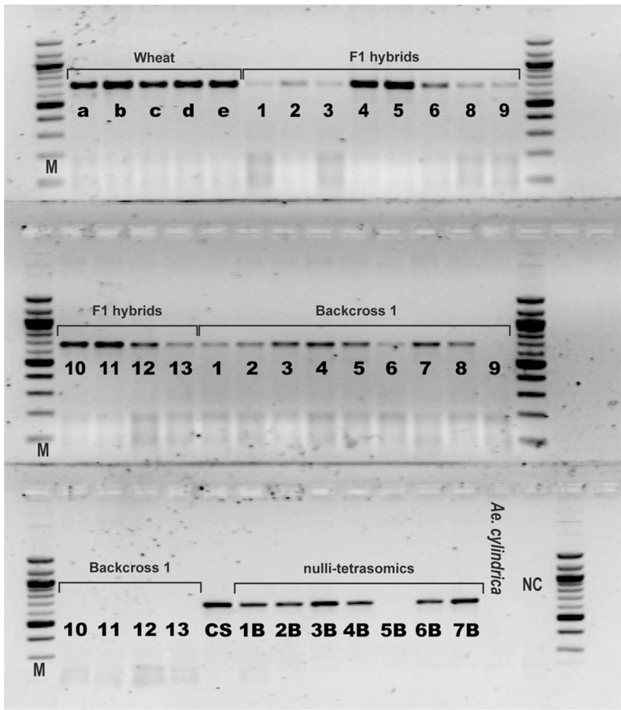
FIGURE 1.- Amplification of the GB10 SCAR marker (662 bp) in wheat (a: Golin 5, b: Greina 16, c: Bobwhite WT, d: Bobwhite 5, e: Bobwhite 8), F1 hybrids, BC1, CS-NT lines and Ae. cylindrica . NC: negative control, M: 100 bp ladder
