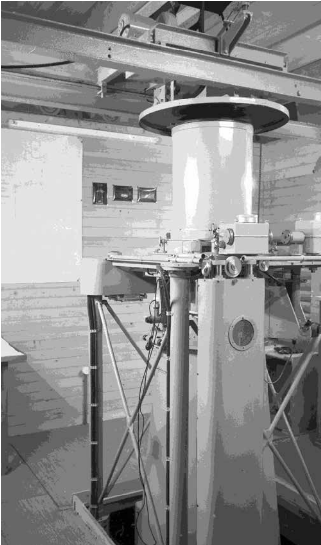
Fig. 4. The PZT of the Neuchâtel Observatory in its context of use. Placed in a hut with two floors. We see here the upper part of the instrument with the rotary and all the devices allowing the photographic recording while the lower part has a mercury bath and the cooling systems of the tube of the instrument. FP-NEG-2859-02.tif © Bibliothèque de la Ville de La Chaux-de-Fonds, Département audiovisuel, Fonds Fernand Perret.
