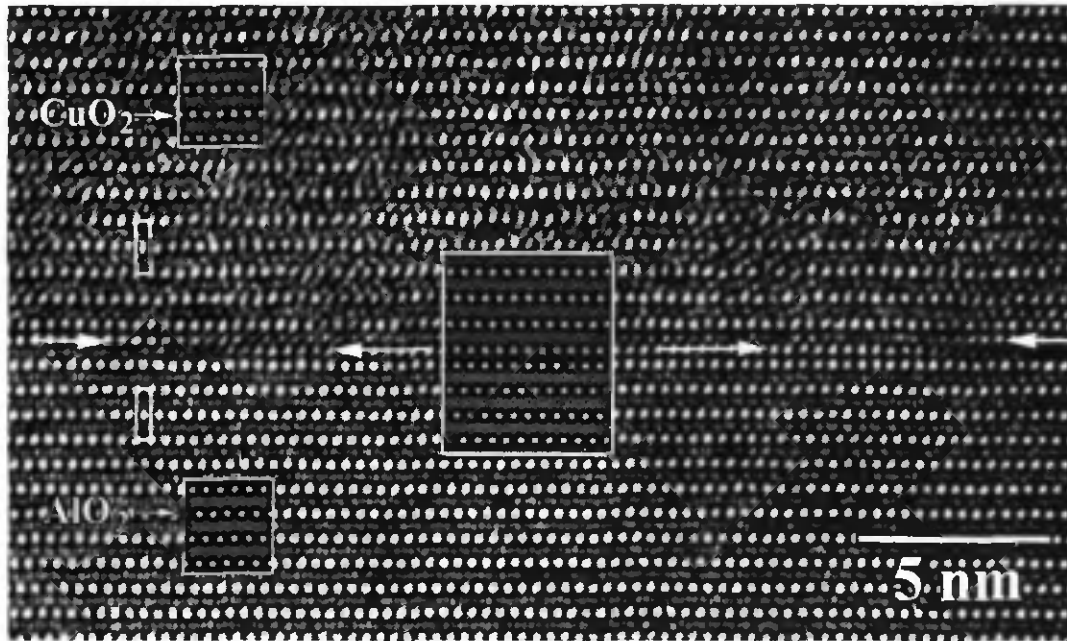
Figure 4. Enlarged HRTEM image of the interface including a simulated image. The bright dots of the image contrast can be correlated with Cu and Al columns in "214" and SLAO, respectively. At the interface, a double row of bright dots occurs, which can be explained by an interface stacking sequence of LaO-AlO 2 -LaO-CuO 2 -LaO leading to an interface structure of (La,Sr) 2 CuAlO 6-x .
