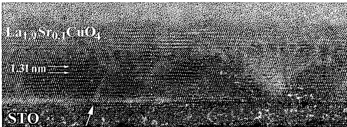
Figure 6. HRTEM image of “214” grown on STO in cross section. The film is not homogeneous, unlike the film on SLAO: it contains planar defects, one of which can be seen in the image and is marked by the large arrow. The planar defects lead to an interruption of \text{CuO}_2 planes; this can be seen as an interruption of the c -axis fringes. The film is 12 unit cells thick, as indicated by the vertical array of dots.
