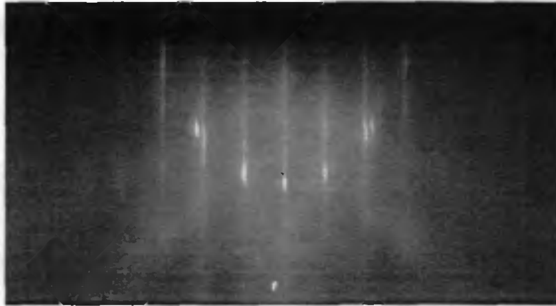
Figure 1. Typical RHEED image subsequent to the deposition.
