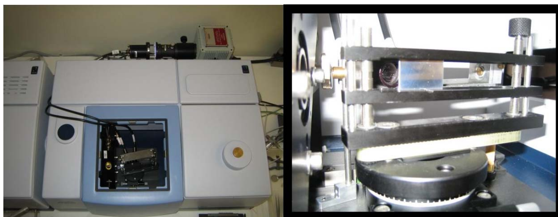
Figure 2-26. PMIRRAS set up on purpose modified for in situ UV exposure. The left hand picture shows the spectrometer external layout (top view) with the optical bundles fixed on the holder, inside the measurement chamber. On the right hand is depicted a blow up of the metallic surface (20x12 mm) installed for simultaneous PM-IRRAS measurement and UV irradiation.
