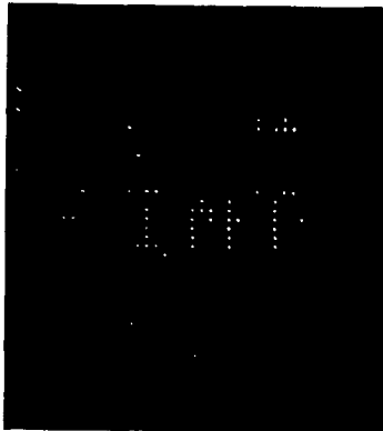
Fig. 4.36 The three letters IMT addressed on a 32 by 32 mirror array.
