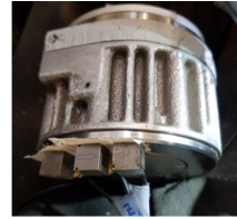
Fig. 1: C axis with accelerometers sensors
