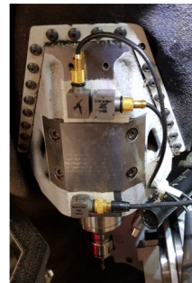
Fig. 2: Spindle axis with accelerometers sensors
