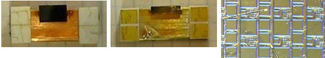
Figure 5.2: Sample pictures. Left: mounted absorption sample. Center: mounted photocurrent sample. The small ceramic pad chip between the two signal contact pads connects a bond from the sample ground to the copper submount by an indium film. The 45^\circ facet is below the long top sample edge. Right: close-up of the mounted photocurrent sample. The ground (bottom) and mesa (top) contact wires are clearly visible. The square mesas have side lengths of 100 \mu\text{m} , 200 \mu\text{m} , and 300 \mu\text{m} .
