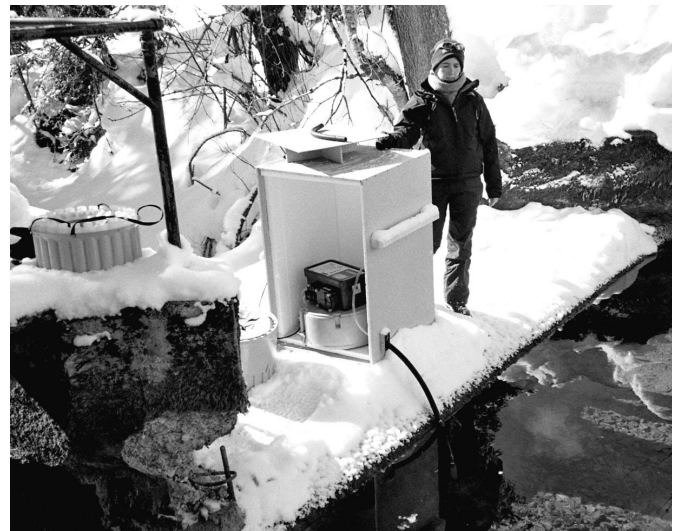
Fig. 2. Automatic sampler at the karst spring that drains the Hölloch cave in the Austro-German Alps (photo: N. Goldscheider). Due to temperatures down to -20\text{ }^{\circ}\text{C} , the sampler was placed into a heated insulated box.
