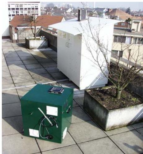
Fig. 4.2. The lidar installed on the 5 th floor balcony of the Institute of Meteorology, Climatology and Remote Sensing in Basel. The lidar is in the dark green box (for protection and transportation), referred as 'lidar unit' in Table 1.2 in Sect. 1.5.2. The white cabinet is an environmental protection for the lidar during the period of measurement.
