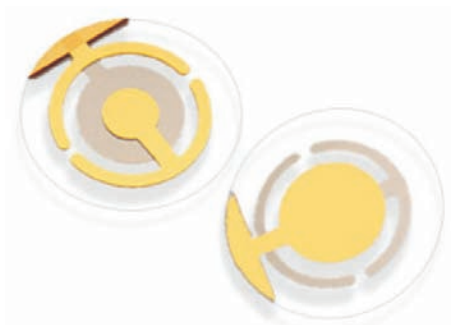
Figure 2.5: AT-cut 1 in. standard QCM sensor crystals. The surface is a chrome/gold composite with an optically clear finish (about 50 nm average surface roughness). The crystal on the left shows the contact surface while the one on the right shows the sensor surface in contact with a gas or liquid.
