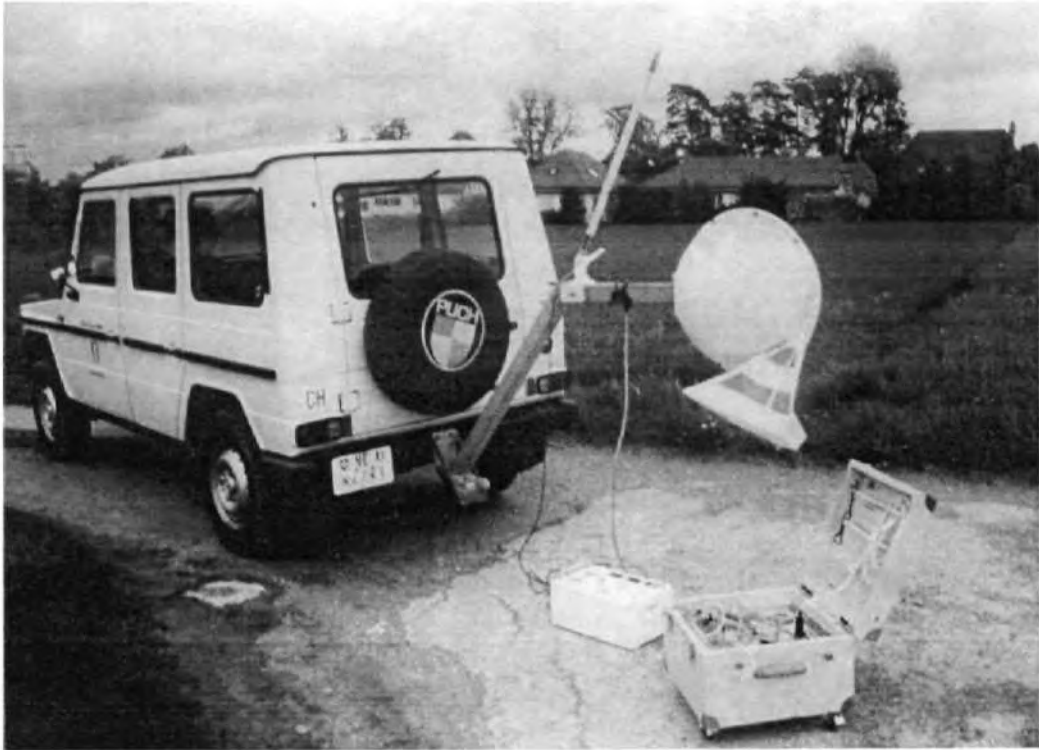
Figure A.12: Electronically oriented antenna (RF-EM 2) fixed behind a car: electrical antenna, plastic balloon with magnetic coils inside, receiver unit, power box
