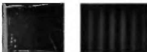
Fig. 2.23: alignment quality of a 200 \mu m wedge-cell obtained with a photo-alignment layer. (a) Between 0° and 90° oriented polarizers (left), (b) regular fringe pattern obtained when placed between 45° oriented polarizers (right).
