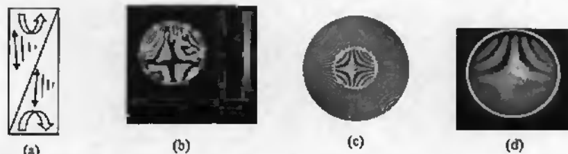
Fig. 7. (a) Schematic of the design with two LC wedges of opposite twist sense. The field of view is simulated by (b) ASAP and (c) LCD Master. (d) Conoscopic observation. The circle has a radius of 35^\circ .
