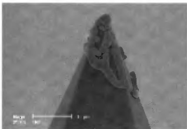
Fig. 4.2. Deposition of electroplated platinum on a not completely open tip shaped electrode.
