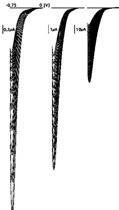
Fig. 3.11. Voltammograms of the platinum deposition.
