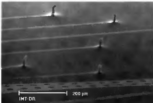
Fig. 3.23. SEM picture of cylindrical platinum electrodes.
