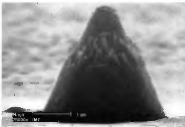
Fig. 3.26. SEM picture of a platinum mini-microtip electrode.
