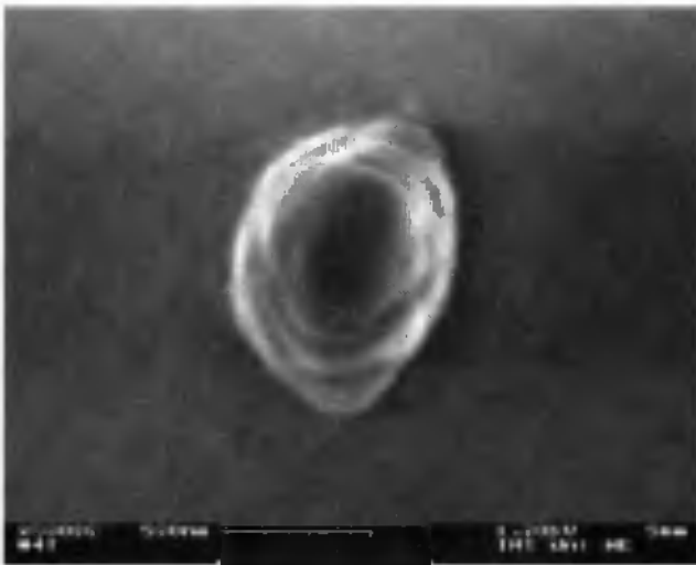
Fig. 3.25. SEM picture of the photolithography performed to achieve the opening of the passivation layer of a mini-microtips.
