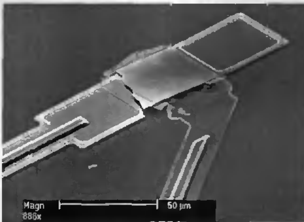
Figure 5.11: Membrane rupture after exposure to humid air and high electric field. It was observed that the cathode corrodes faster.
