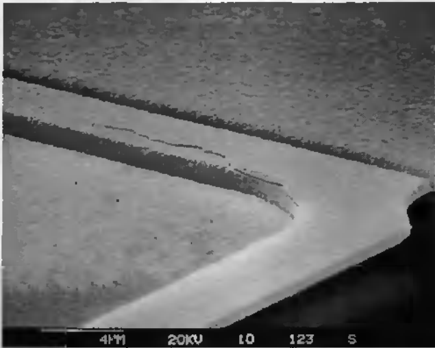
Figure 5.5: SEM micrograph of a precracked polysilicon membrane. Such test-structures are used to measure the crack-growth rate.
