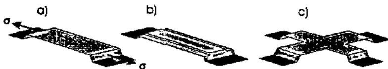
Figure 3.15: Design variations for an increased resonance frequency and maintaining a critical damping. a) Internal tensile stress, b) increased beam stiffness by profiled beam, c) clamping at more than two points.
