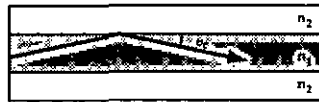
Figure 5.1: A dielectric waveguide is composed of a core with an index of refraction n_1 and a cladding with a refractive index n_2 . A light beam inside the core will be totally reflected at the interface if n_1 > n_2 and if its angle of incidence \theta \leq than a critical angle \theta_c .
