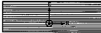
Figure 2.2: To couple light with ISB quantum wells, the electric field vector must be normal to the layer.
