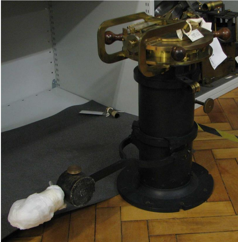
The top section of Airy's Reflex Zenith Tube. Photo taken in the Science Museum storage in 2009
