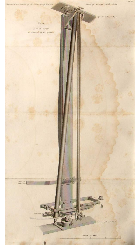
Bradley's Zenith Sector following the modifications made prior to sending it to the Cape in 1837. Plate XV from Volume 1 of Verification and extension of La Caille's arc of meridian at the Cape of Good Hope (1866)
