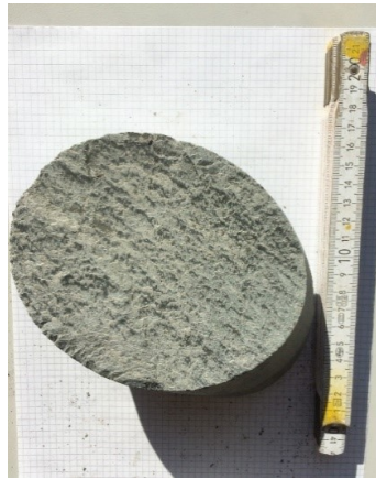
Figure 2.6: NNE-striking fault plane
