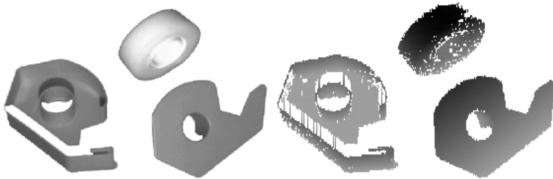
Fig. 4. Intensity and z-image of a typical robot workspace
