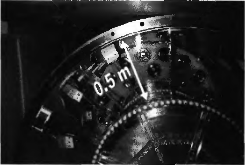
Figure 2.7: The space between the TPC and the steel tank, the acrylic tubes to sustain the TPC and the photomultipliers to detect the scintillation light
