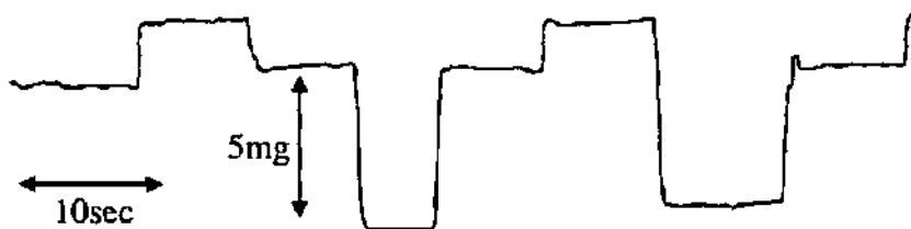
Figure 4.47: Accelerometer response to various static accelerations steps.
