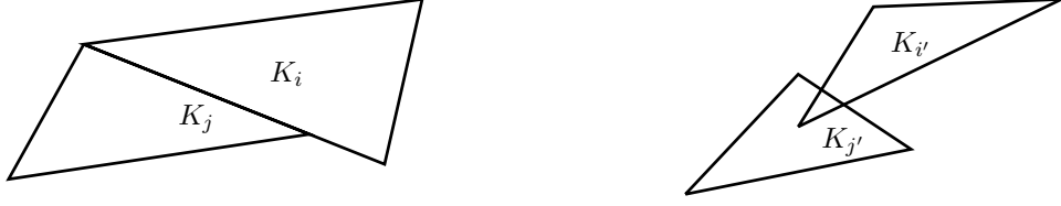
Figure 2.1: The couples of 2-simplices (or triangles) \{K_i, K_j\} and \{K_{i'}, K_{j'}\} does not satisfy the condition (v). Moreover, the couple \{K_{i'}, K_{j'}\} does not verify (iv) neither.
