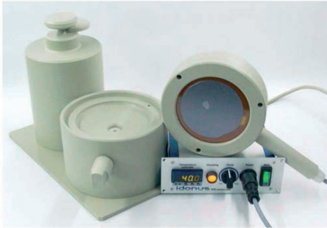
Figure 3.13 : Experimental set-up used for the hydrofluoric acid (HF) vapor phase etching (VPE). The components are: the wafer holder with an integrated heating element, the reaction chamber containing liquid HF (49%), the feedback system used to control the temperature of the wafer holder, and a saleable container dedicated to the storage of used HF or to the refilling of the process chamber.
