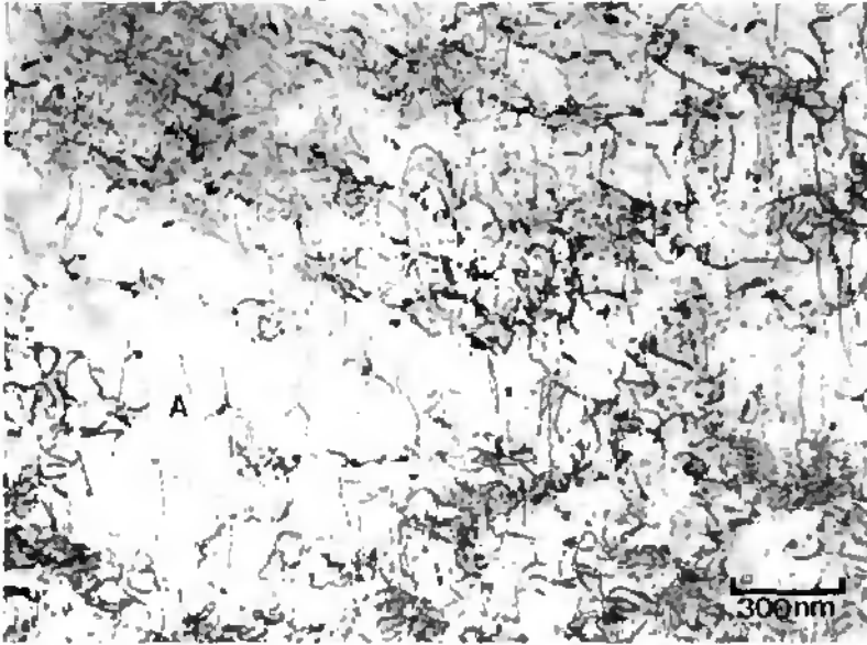
Fig. 4-29 Deformed microstructure upon forging at 400°C showing high density of dislocation
