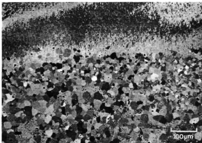
Fig. 4-21 900°C Forged and slow quenched microstructure ( about 5 seconds after forging before quenching )
