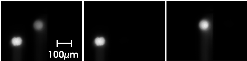
Figure 6.18: CCD images corresponding to the image plane of the spectrometer. In the first image, two objects are present in the field of view, in the second and third image one out of two object is selected, blocking completely the light of the other object. The projected object has a diameter of 50\mu\text{m} which corresponds to the size of a typical astronomical object in the focal plane of a telescope.
