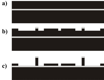
Figure 5.2: Electrode chip fabrication process sequence. As starting substrate a SOI wafer with a 50\mu\text{m} -thick device layer ( 35\mu\text{m} for MIRA2) is utilized (a). In a two-level DRIE process (delay mask process [27]) the electrodes (lower level) and spacers are etched into the device layer. In a first step the patterns of the lower level are etched utilizing a resist mask(b); at this time the height of the electrodes is defined through timed-etching. Then the resist mask is removed and the pattern is transferred to the bottom of the device layer, such that the trenches between the electrodes are completely etched and provide electrical insulation. The spacer structures are protected during the two etch steps with an oxide mask, so that the resulting spacers have the height of the initial thickness of the device layer. After completion of the delay mask process the chips are singulated either by dicing (MIRA1) or a dice-free release process, involving an additional DRIE of the backside and HF vapor release (MIRA2).
