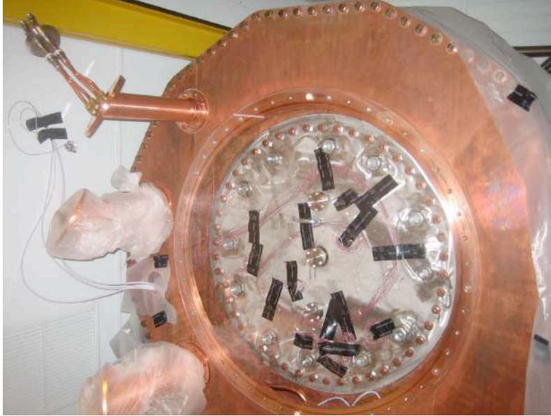
Figure 2.6: Copper cryostat installation in the cleanroom.
