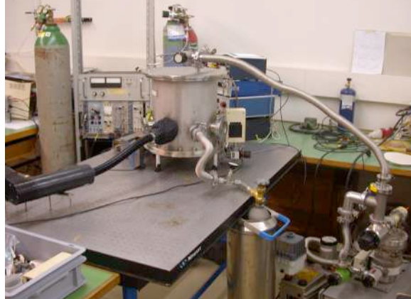
Figure 4.11: Technical drawing of the experimental setup (left). Custom made TPC for SILEM and scintillation light tests (right).
