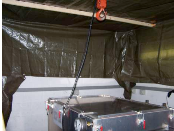
Figure 5.2: Germanium protection against dust.
