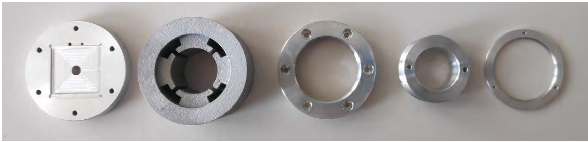
Figure 4.10: Left to right: cavity bottom with grating insert, additive manufactured electrodes part and top part.
