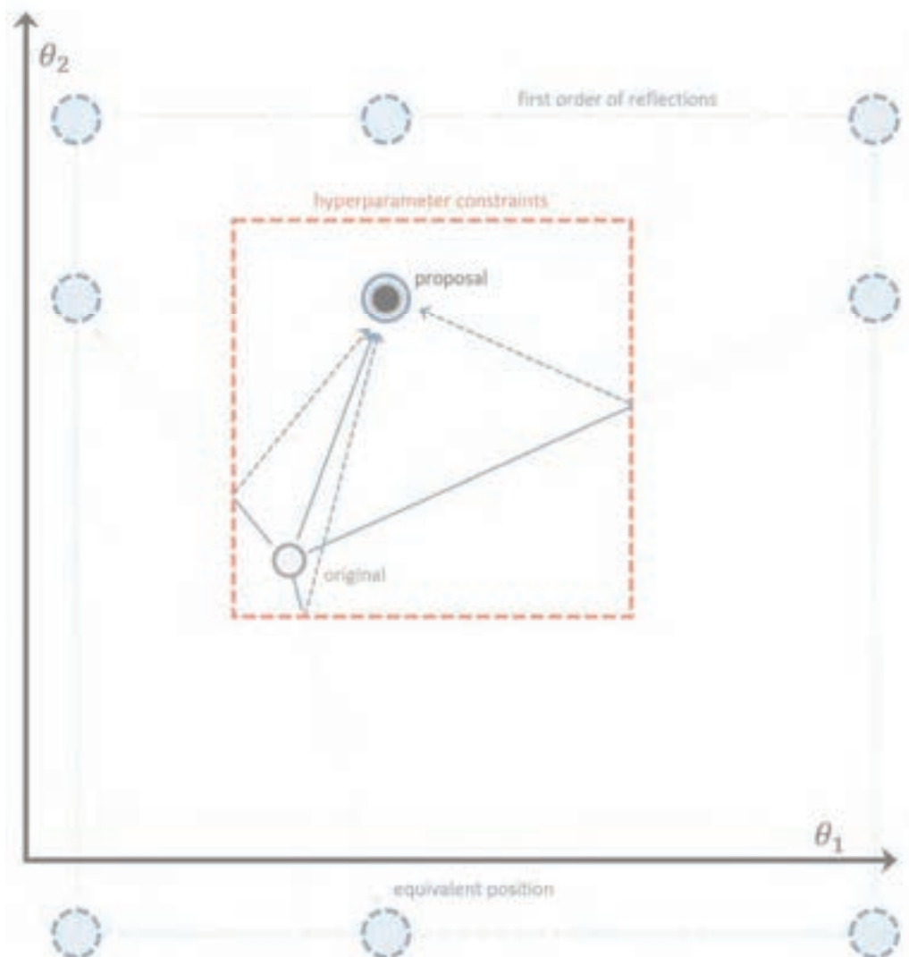
Figure II-2. Equivalent positions (dashed blue circles) to the proposal (full blue circle) along two hyperparameter space dimensions with an upper and lower limit each (red dashed rectangle). Jumps to any of the equivalent positions result in the same proposal after reflection over the hyperparameter constraints.
