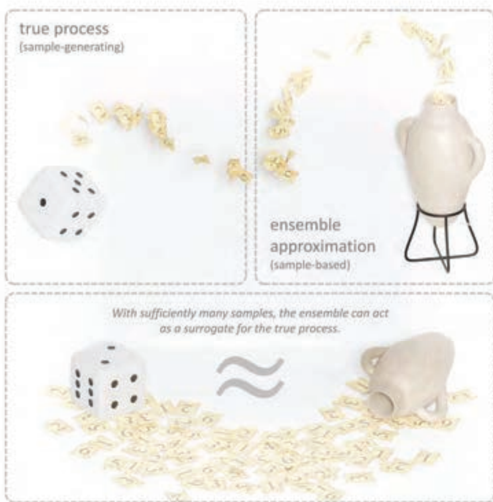
Figure 1-6. Schematic illustration of a Monte Carlo approximation. After drawing sufficiently many samples from a pdf or a random process, the collection of samples (ensemble) may act as a surrogate for the true process or pdf.
