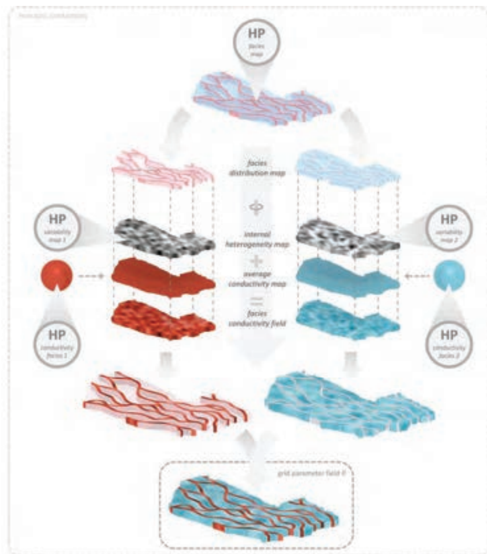
Figure 3-4. Schematic render of the field generator. We generate facies conductivity fields for the background sediment and paleo-channels by offsetting a uniform, average conductivity field with internal variability. The facies distribution map then extracts grid parameter values from each map according to the facies assignment and assembles the parameter field \theta . Assignment of specific yield proceeds equivalently, barring the addition of internal heterogeneity.
