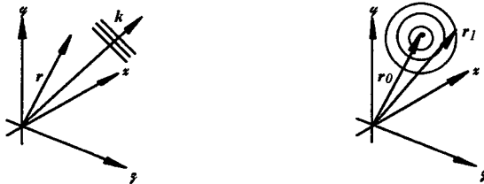
Figure 2.2-2: Two possible solutions of the homogenous scalar Helmholtz equation: left the plane wave, right the spherical wave.
