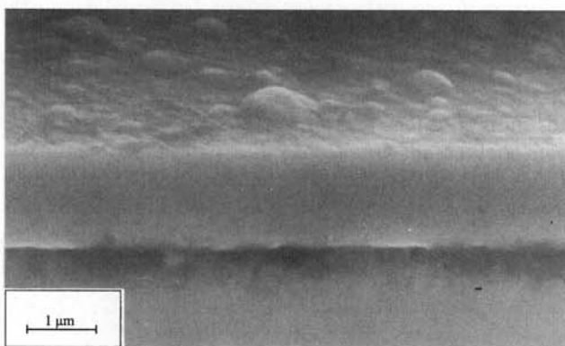
Fig. 1. SEM image of a 1 \mu\text{m} thick DLC film on crystalline silicon.
