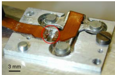
Figure 2.21: Backside view of the platform. The flexprint had been cut at the interface and wire bonding had then been employed for reconnecting the copper lines.
