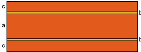
Figure 2.35: Schematic cross section of the flexprint PCB. a) Kapton layer, thickness 50 \mu\text{m} . b) Copper lines, thickness 15 \mu\text{m} . c) Kapton layers, thickness 25 \mu\text{m} . This symmetrical design avoids the bimorph effect.
