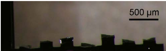
Figure 4.45: Image of the base of the beams after their removal by the cleaving tool. The position of breaking varies from one beam to another.
