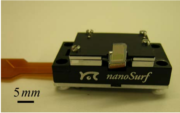
Figure 2.43: The AFM scanner of the second generation with an AFM chip mounted on it. The external dimensions of this scanner and its weight were kept constant compared to the model of the first generation.
