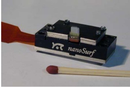
Figure 2.18: Front view of the AFM scanner (first generation) with a mounted AFM chip. The scanner had an overall size of 24mm x 18mm x 12mm and weights only 15g.
