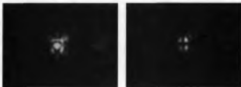
Figure 7.12: Emission pattern of an elongated aperture structured on a square quartz tip. The left image is the field component polarized parallel to the incident beam polarization (x-axis) and the right image is the component along the y-axis.
