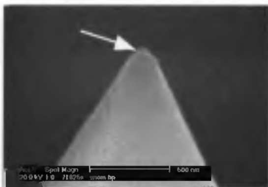
Figure 6.8: SEM photograph of a tip after selective etching of the nitride. The tip apex is still covered with aluminum.
