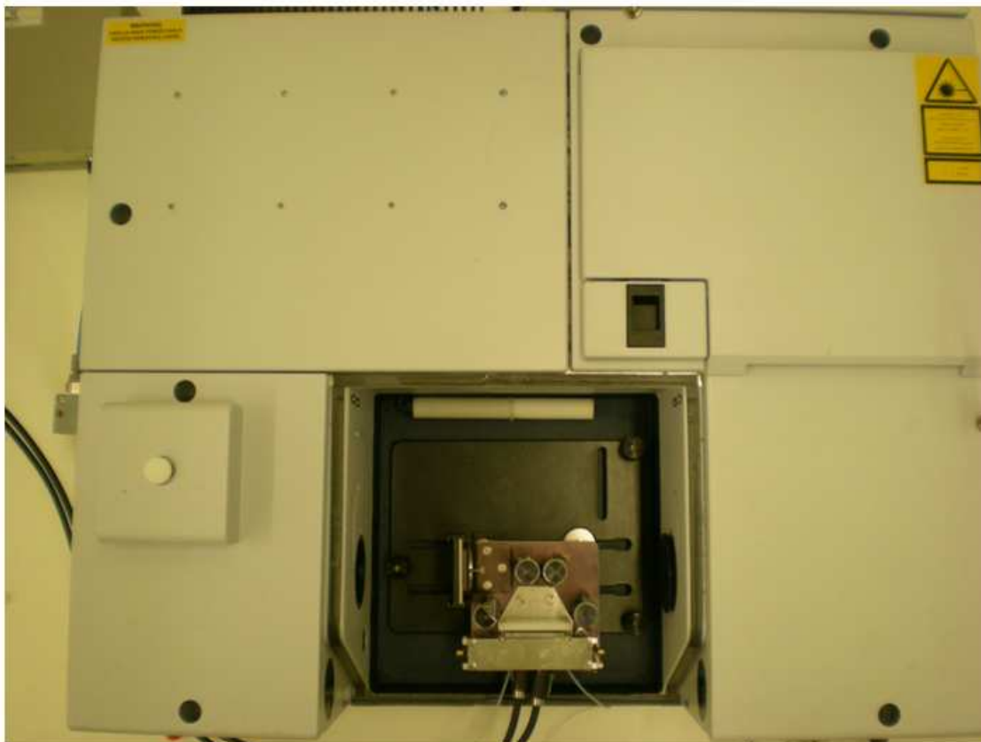
Figure 2-2: The Bruker Equinox 55 ATR-IR spectrometer equipped with ATR-IR attachment and flow-through cell for in situ photocatalytic measurements.
