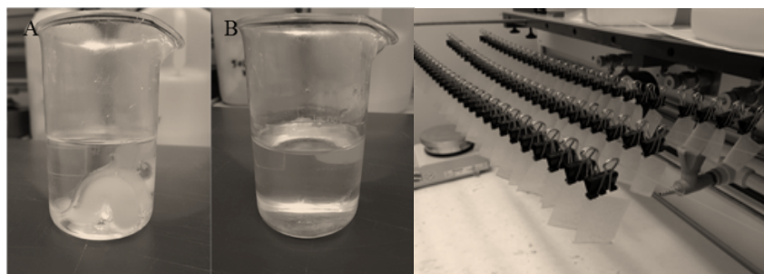
Figure 9. Silicone glue before (A) and after (B) dissolving in toluene. Squares of lens paper are dipped into solution B to prepare membranes. Right: The drying line used for air-drying membranes in a fume hood consisting of fishing line and binder clips.
