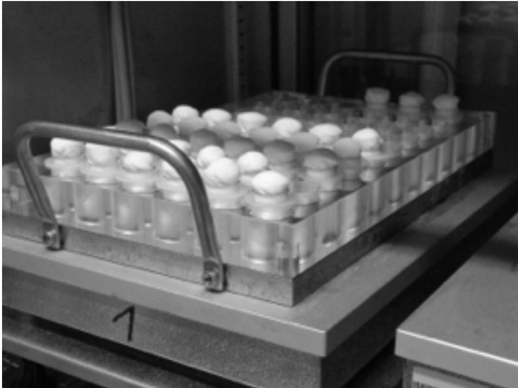
Figure 12. Plexiglas ® feeding unit holder with feeding units on top of steel 60-well plate containing blood, and hot plate.
