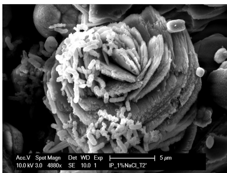
Figure 4: Scanning electron microscopy image taken during our experiments and showing the formation of iron phosphate minerals as by-products of the reduction of insoluble Fe(III) oxides by Shewanella loihica .
