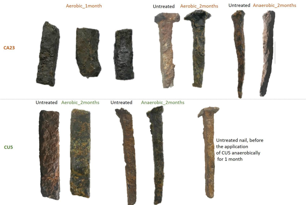
Figure SI10: Visual observations of archaeological iron objects before and after treatment with CA23 and CU5. These are the photos of the objects treated (Aerobic and /or Anaerobic) and before treatment (untreated). This figure represents the remaining results that were not presented in Fig. 6.
