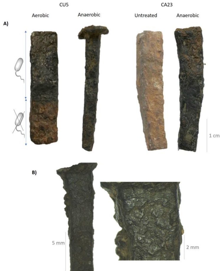
Figure 6: Optimised bacterial treatment on archaeological iron objects. A) Visual aspect of the iron nails treated with the bacterium CU5 (aerobically and anaerobically) in comparison to the abiotic control (gel delivery system without the bacterium) and CA23 (anaerobically) in comparison to the untreated after 1 month of incubation. B) Spectroscopic images of an archeological nail treated with CU5 anaerobically after 2 months of incubation.
