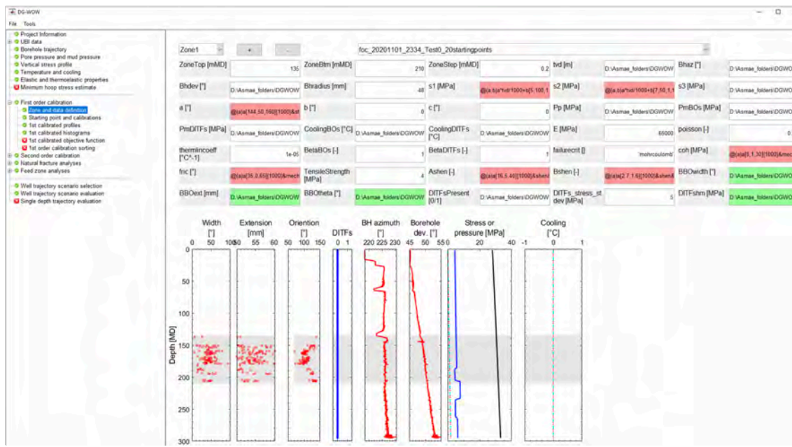
Figure 7.4.: Screenshot of the "Data and Zone Definition" panel of the DG-WOW-app when testing it on the CB1 borehole. One zone was defined in this example where calibration will be performed as well as the required data such as static parameters (white boxes), observations (green boxes) and parameters to be estimated (red boxes). The shaded grey area in the lower part of the panel depicts the zone of calibration (135-210 m MD in this example).
