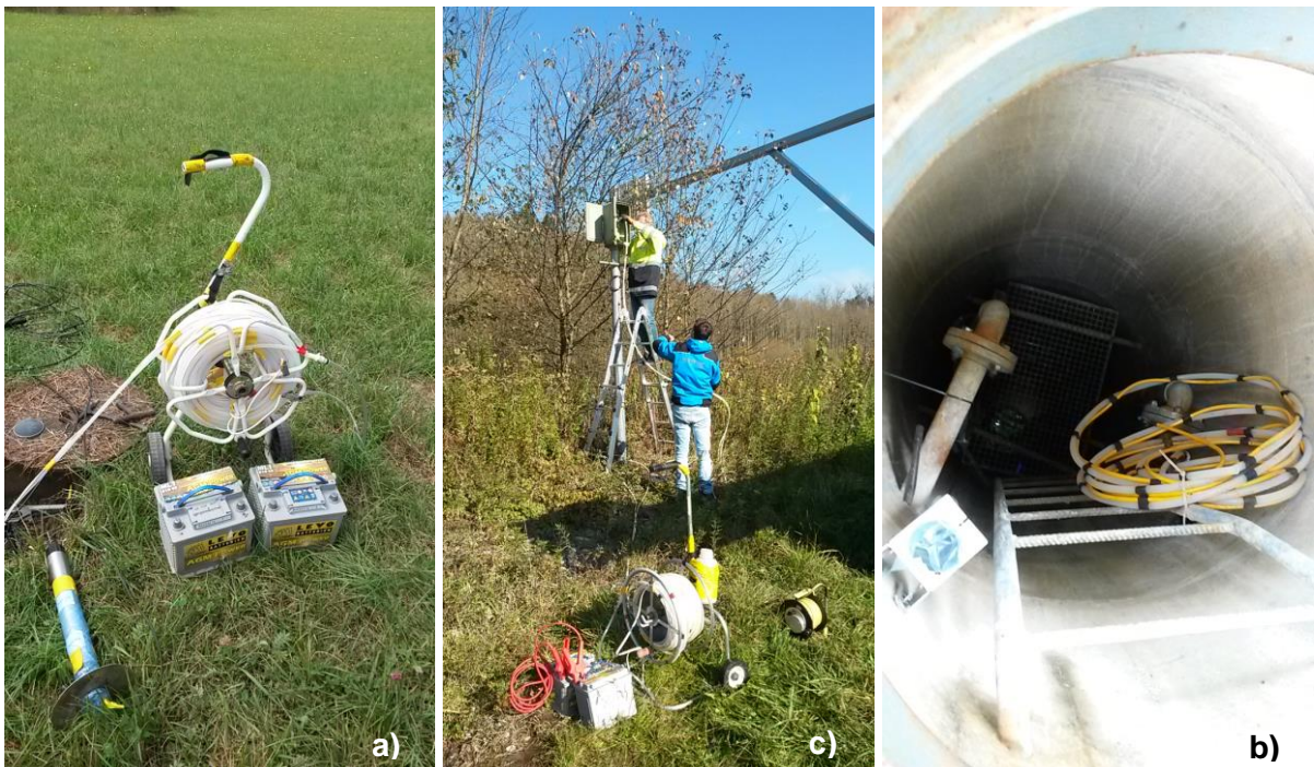
Figure 1-3: Groundwater monitoring wells along the Thur River range from a) regular monitoring wells installed at ground level, b) boreholes with elevated casings to protect loggers from floodwaters, c) large-diameter borehole.
