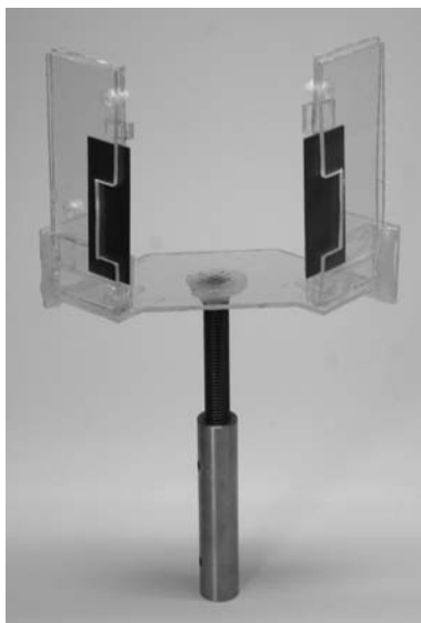
Figure 4.13.: This holder is the development of figure 4.12. The advantage is that this holder has two objects (sheets) fixed, selectable with the rotation stage.
