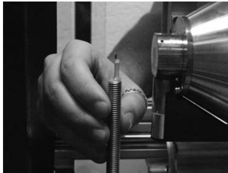
Figure 3.21.: Sample holder with a sample of a bee brain in front of the X-ray source.
