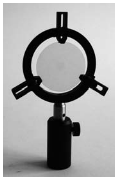
Figure 3.17.: A free standing scintillator based on yttrium aluminum garnet (YAG) doped with cerium. The thickness is 300 \mu\text{m} .
