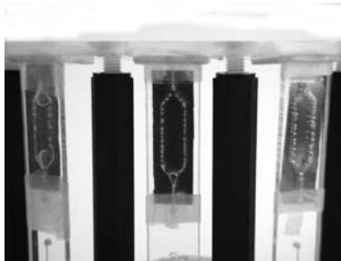
Figure 4.29.: Filled cuvette fixed in the holder. Behind the cuvette a titanium sheet of 23 \mu\text{m} is glued. In the liquid air bubbles are visible. Both holes of the cuvette are sealed to avoid liquid evaporation.
