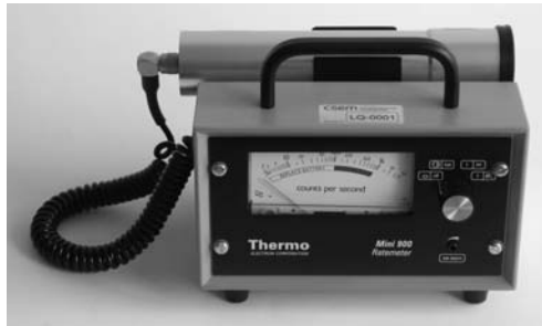
Figure 3.3.: For the measurement of the radiation level outside of the shielding a ratemeter from Thermo is used.
