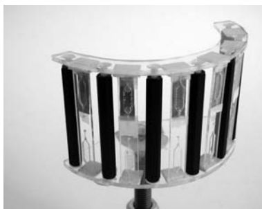
Figure 4.16.: Holder with 6 cuvettes for measuring multiple liquids at one time.
