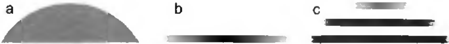
Figure 2.2: Approximation of a real lens (a) by the thin element approximation (b) and the beam propagation method (c).
