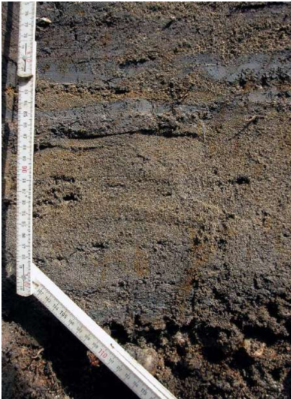
Fig. 4.23. View of the bottom layers of soil profile 6 showing various textural layers.
