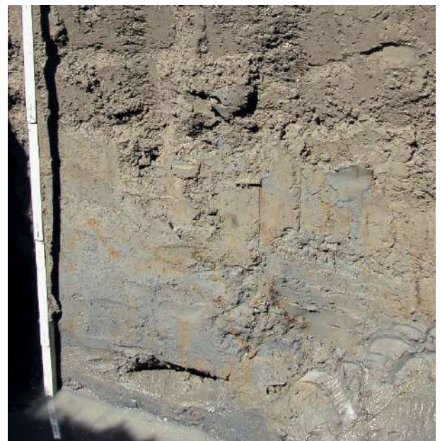
Fig. 4.41. View of the bottom layers of soil profile 13 showing coarse deposits, as well as a fluctuating water table.
