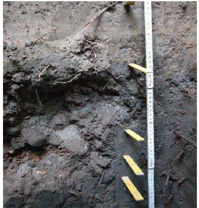
Fig. 4.25. View of gravels and coarse material found between 80 and 95 cm in the soil profile 7 indicating a high flow discharge flood in the middle of the profile.
