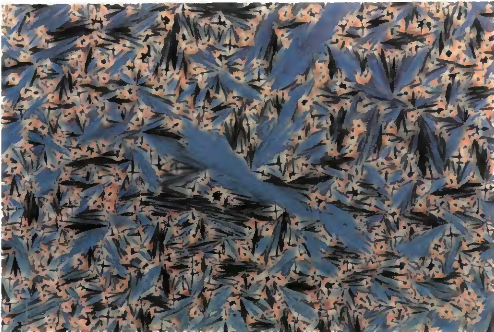
Fig. 4. Representative thermal polarized optical micrograph of the focal-conic texture displayed by III ( n = 12 ) in the smectic-A phase upon cooling from the isotropic liquid to 164^\circ ( 200\times )
