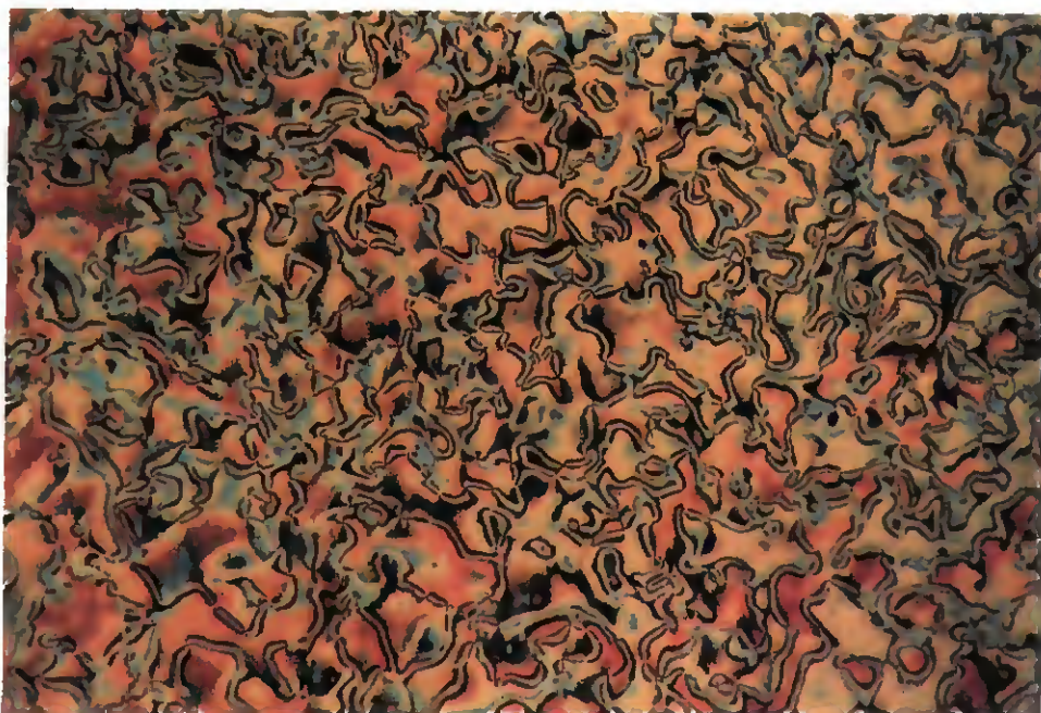
Fig. 2. Representative thermal polarized optical micrograph of the smectic C Schlieren texture displayed by 1n ( n = 14 ) upon cooling from the nematic phase to 168^\circ
