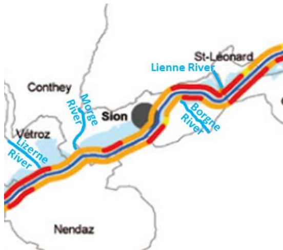
Figure 1.3: The discharge capacity of the Rhône River in the study zone [Canton du Valais, 2016], located in Figure 1.1 . Blue lines represent the major rivers. Light Blue areas represent inundation zones. The red, orange and yellow lines along both sides of the Rhône River showed its hydraulic capacity: Red : inferior to Q_{100min} ; Orange : between Q_{100min} and Q_{100cible} ; Yellow : superior to Q_{100cible} .
