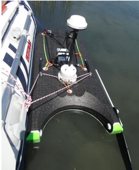
Figure 4.12: Acoustic Doppler Profiler mounted on a float geolocalised by GPS and moved with an electric boat.
