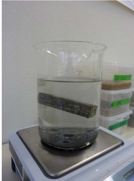
Figure 7-4 Rock sample immersed in deionized water during a density measure.
