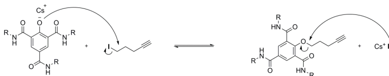
Scheme 17. Possible mechanism of ether cleavage of 2-alkoxy-BTA derivatives.
