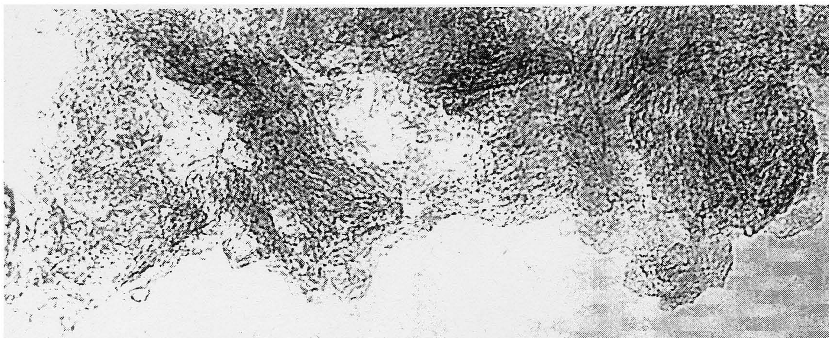
Figure 6 High resolution electron micrograph of carbon U. Final magnification of 1,500,000 \times (Philips EM-300, underfocussed 80 nm approximately).
