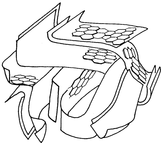
Fig. 1. A schematic representation of the microstructure of active carbons.
