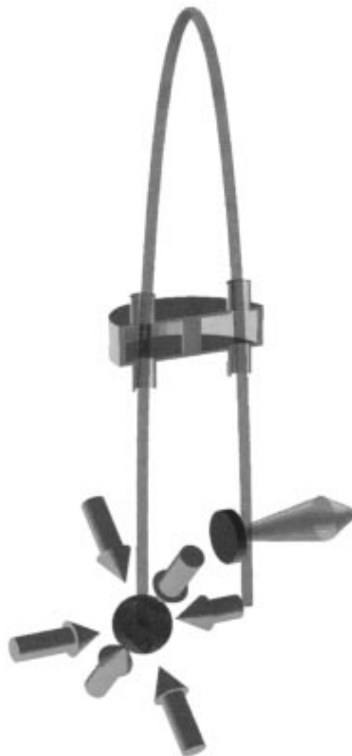
Fig. 1. Basic configuration of the continuous fountain, showing the six cooling beams, the microwave cavity and the detection region.
