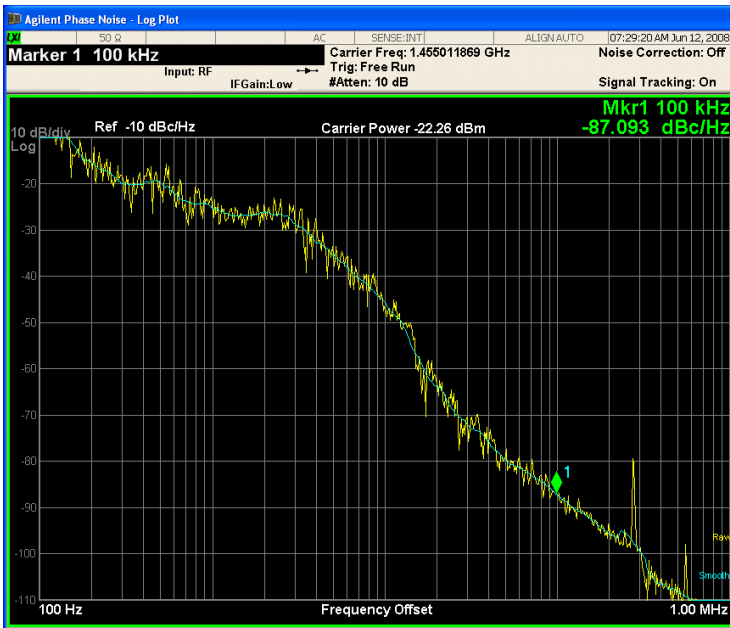
Figure 7.47: The measured output phase noise of the PLL.
