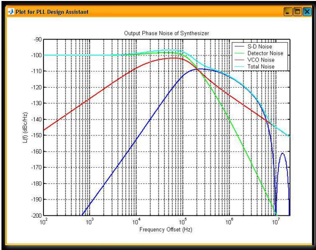
Figure 7.26: Simulated PLL output phase noise with 120 kHz loop bandwidth.
