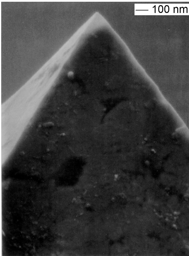
Fig. 5. SEM image of the apex of a pyramidal diamond tip
