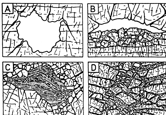
Fig. 5.15 – Types of filling of karst channels. A – open karst channels; B – karst channels partly filled with breccia zones; C - karst channels filled with fine-grained sediments; C – breccia zones. Adapted from Adamczyk et al. 1988.
