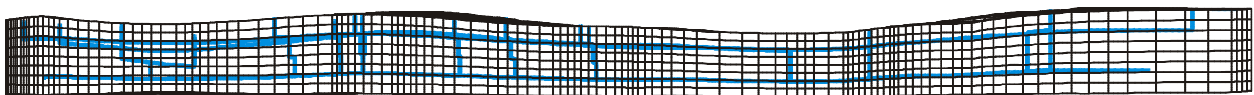
Fig. 6.5 – 3-D finite element mesh, after the definition of altitude for each node.
